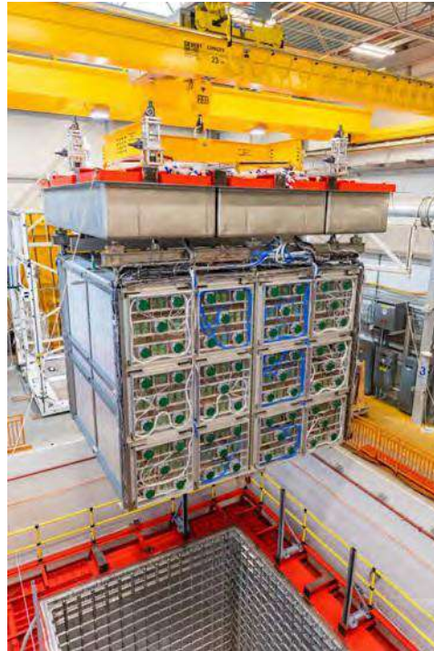
Rigging detector into cryostat
