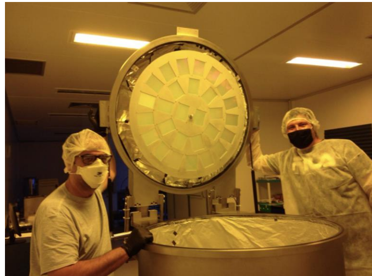
1400 Short pass dichroic filters Produced by OPTO company (Brazil) – ProtoDUNE HD and VD
